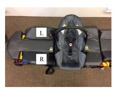
C. Feed the stretcher shoulder belt male and female ends through car bed webbing loops at the head of stretcher.
